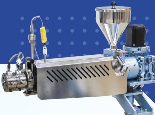
Compact, high-precision single-screw extruder for laboratory-scale testing, compounding and filament production.
