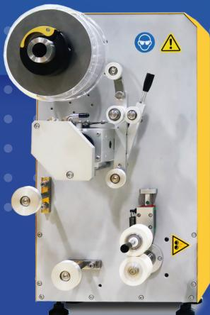
Designed for collecting continuous filaments or extruded profiles with controlled winding, the system combines rubber pull rolls, a strand guide assembly on a traverse unit, and a servo-driven winder to coil filaments onto the reel.
