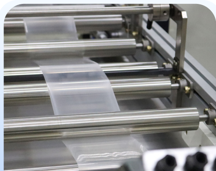
Stainless-steel guide rolls for precise film alignment and easy cleaning.
