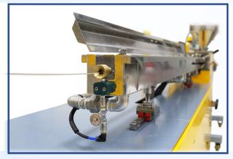
The tank exit is equipped with an air wipe assembly to effectively remove moisture and ensure proper drying of the filament before winding it up on the spool.
