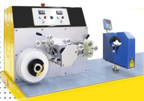
The Traverse Spool Winder Station features a pair of urethane pull rolls and a traversing strand guide that directs the filament onto the loaded spool driven by a servo motor.
