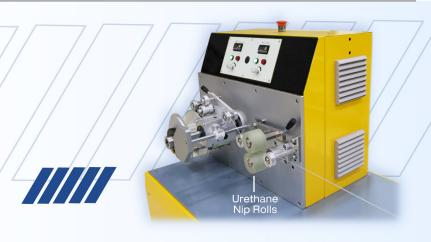
The pull roll grips the filament and draws over the grooved guide rolls until it is wound to the spool via the strand guide. The strand guide is mounted over an adjustable traversing unit equipped with mechanical traverse drive motor that oscillates along the inside width of the spool, for a tight and even filament winding distribution.
