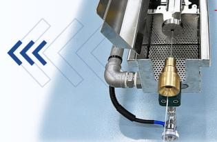
The tank is fitted with a stainless-steel sizing tool at both ends to maintain the proper alignment and shape stability of the filament being steadily drawn along the guide-trough. It also functions as a flood seal to prevent water leaks.
