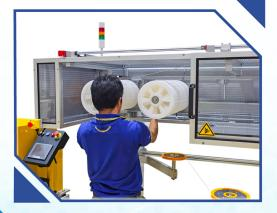
The filament is alternately guided through the pulleys. During the spool changeover at the winder, the filament accumulates continuously as the shaft with many pulleys moves sideways to facilitate continuous and uninterrupted operation.
